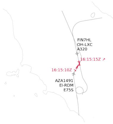
Fig. 17. Flight paths of FIN7HL and AZA1491 above Italy. Parts of path marked in red indicate distance covered during a TCAS RA.
